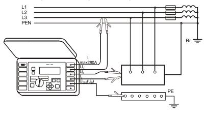
Fig.18. Measurement of touch voltage U<sub>ST</sub>
