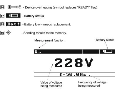
Fig.2. Screen layout in alternating voltage measurement mode
