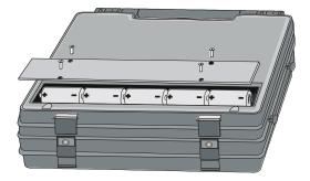
Fig. 8. Opening the battery compartment
