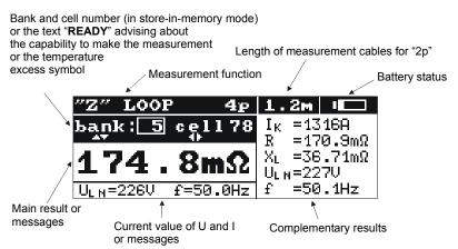
Fig.3. Screen layout in short-circuit loop impedance measurement mode (all results)
