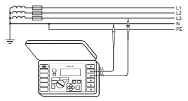
Fig.9. Alternating voltage measurement
