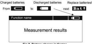
Fig.7. Battery charge indicator
