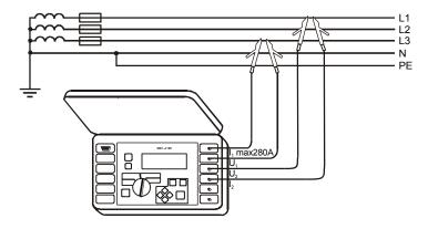
Fig.15. Measurement of impedance in working circuit (L-L) using four-pole method
