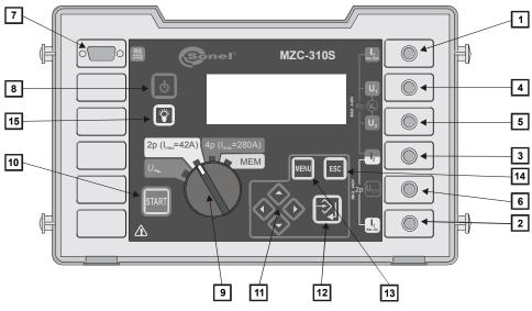
Fig.1. MZC-310S front panel layout
