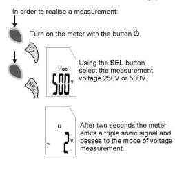
Connect the terminals of the meter to the object being measured.
