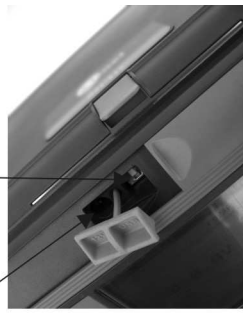
Meter power supply ON/OFF button MENU - selection of additional meter settings Display backlight ON/OFF button
