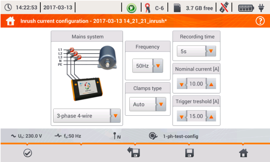
Fig. 35. Inrush current configuration screen.
