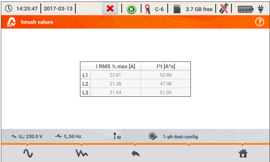
Fig. 40. Inrush current - characteristic parameters.
