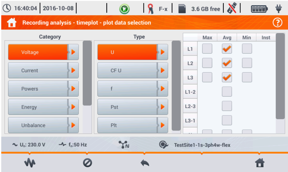
Fig. 23. Recording analysis - selecting parameters for the timeplot.
