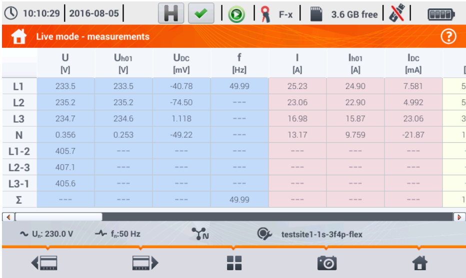
Fig. 43. Live mode – measurements results table.
