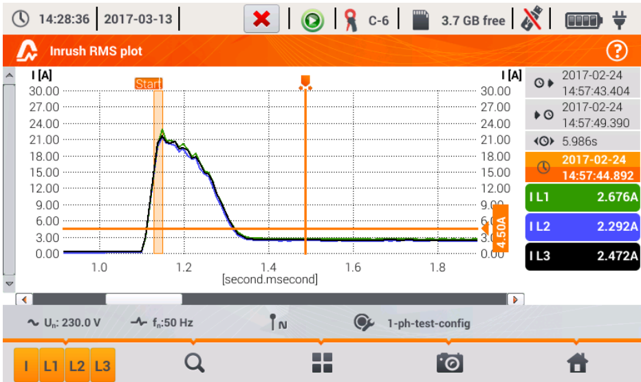
Fig. 39. Inrush current analysis – Inrush RMS plot.
