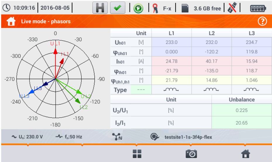
Fig. 44. Live mode – phasor diagram.
