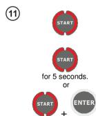
Press and hold **START** push-button. The measurement is performed continuously until you release the button or the pre-set time is reached.
