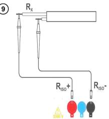
Connect test leads according to the drawing.
