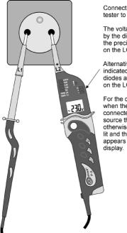
Connect both probes of tester to the live object.
